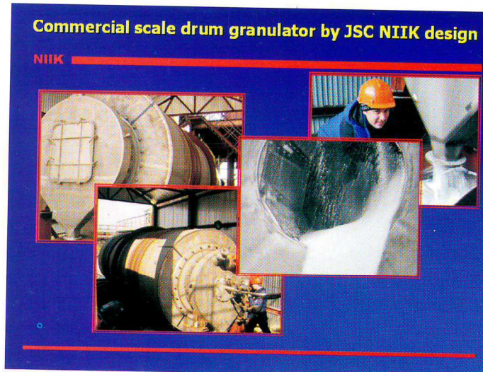
Picture 6. Drum granulator by JSC NIIK design successfully integrated with existing urea unit.
