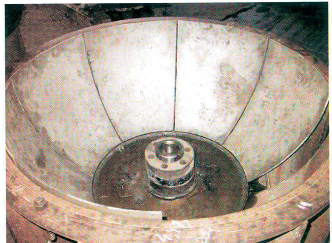
Picture 4. Jigging tool developed by JSC NIIK for relining of spherical parts of vessels
